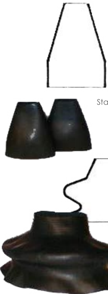
Bellow neck seals allow for more head movement without ingress of water
