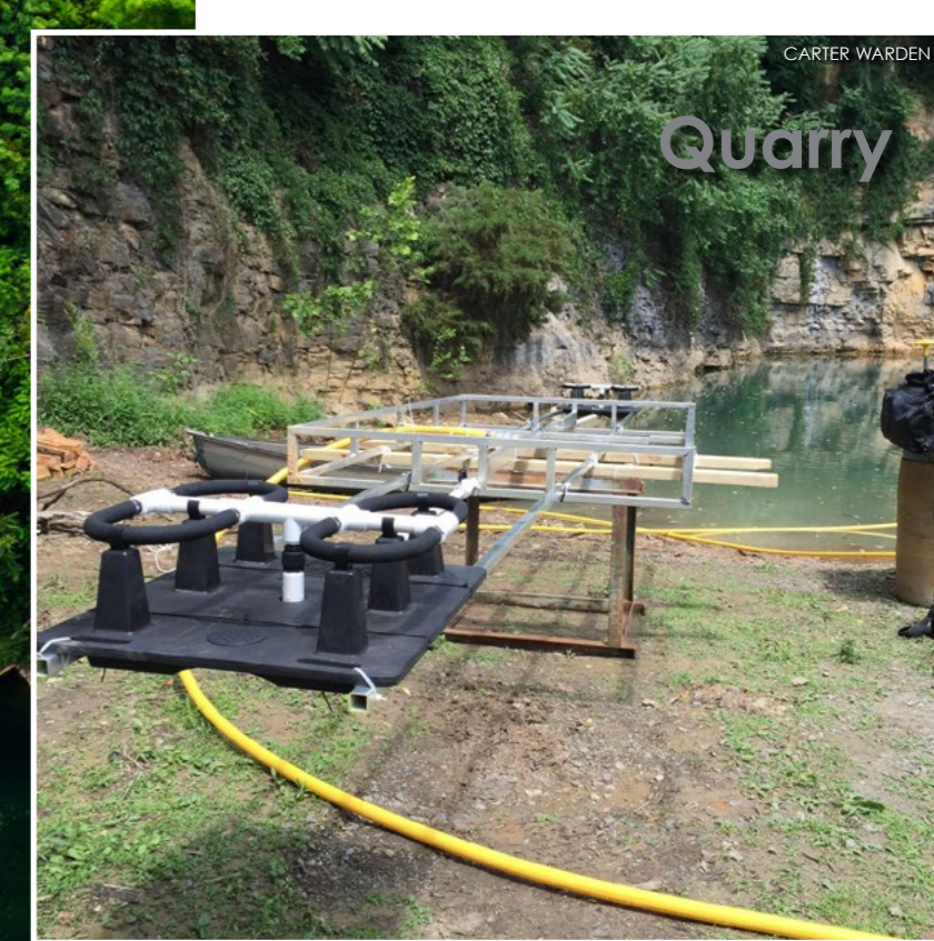
Aerator assembly, showing hose (above); Further improvements to Gray quarry included a staging area for divers with picnic tables, tank stands, changing area and floating platform with submerged stairs (left).
