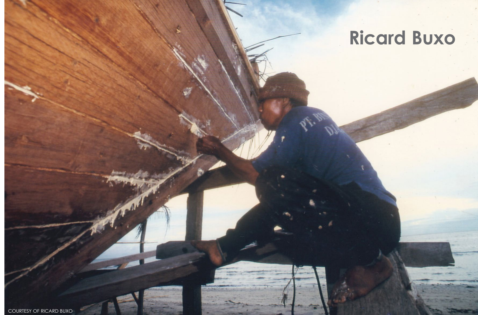
Laying the main deck of the Ondina (top left); Sealing the hull (top right); The pinisi under construction at Tanah Beru (right); The lounge and dining area under construction (left)
